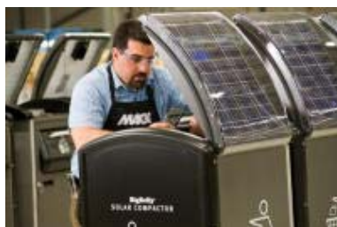
Chris Glaski, Mack metals engineer, tests the wireless monitoring system that signals when the solar compactor is full, allowing managers to optimize collection efficiency on a real-time basis. (Courtesy Mack Molding)
