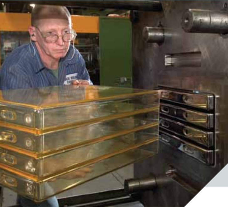
The energy market is booming for Mack Molding. Pictured is battery cell molding.
