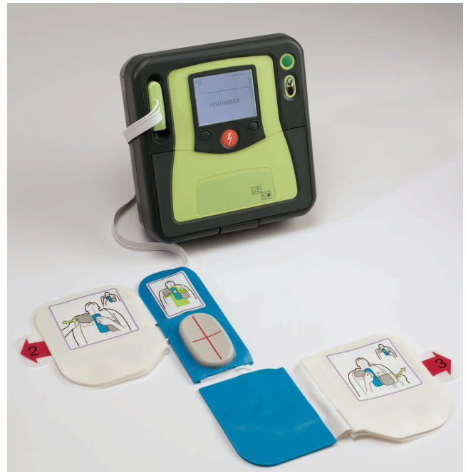
Figure 7. This AED from Zoll Medical (Chelmsford, MA) was made with overmolded soft-touch materials.
