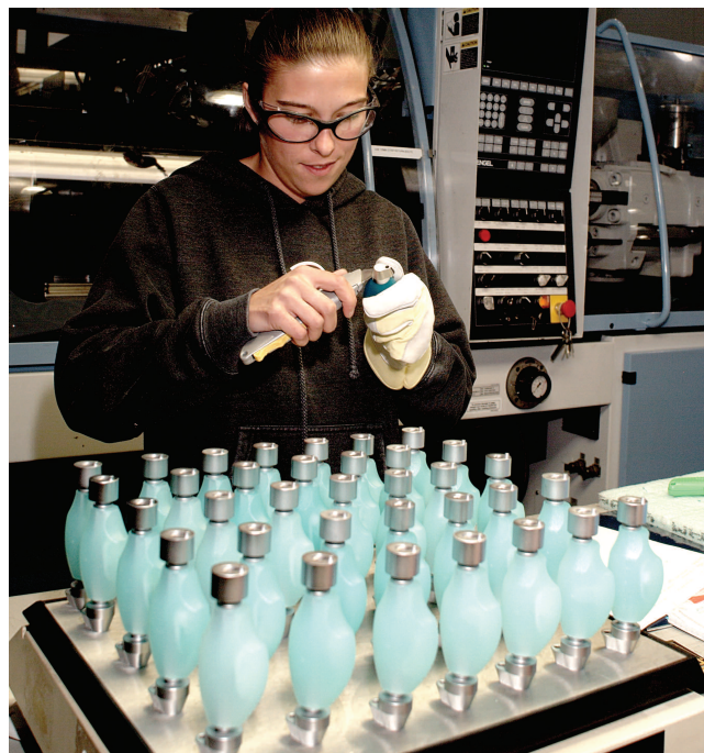
Figure 3. At this press, both the substrate material and soft-touch overmold for surgical instrument handles are molded in two subsequent processes.
