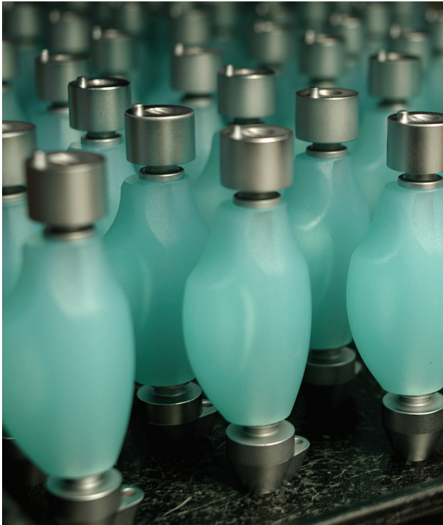
Figure 4. The substrates for the handles before the soft-touch overmolding. The design of the handles required two overmolding processes to produce the final part.
