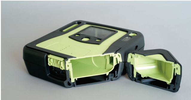
Figure 8. A cross section of a Zoll AED clamshell illustrates the overmolded gas-assist features of the device.
