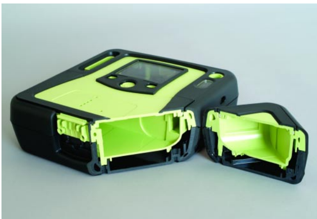
Figure 10. The gas channels ensured that the gas hollowed out and packed the base of the bosses on a clamshell for Zoll.
