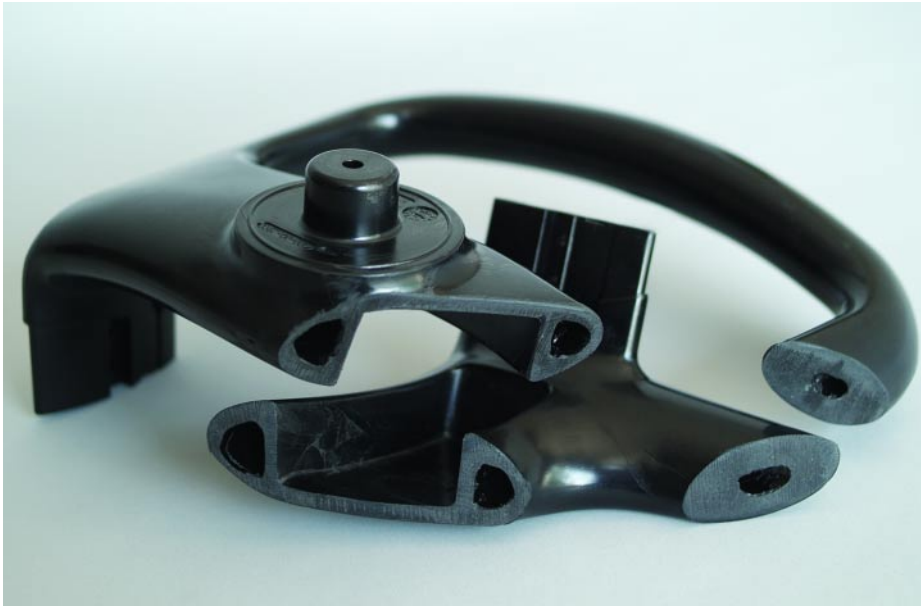
Figure 8. To make a Datascope main handle, a number of gas nozzles were timed to control the introduction of the gas in different locations.
