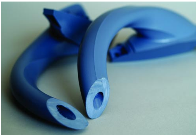
Figure 6. Using gas-assist molding ensured consistent wall thicknesses over the length of Alcon’s Infiniti main handle.
