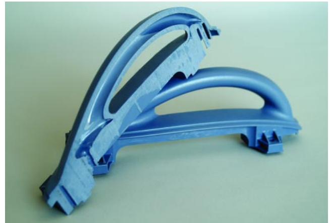
Figure 7. The gas evenly hollowed out the Infiniti’s side handle. It is a closed-loop part, so overspill technology was required.
