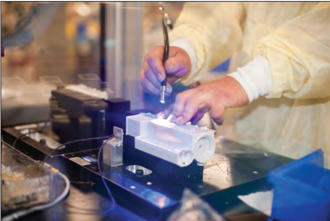
Fig. 2 – Mack installs functional lenses in the disposable patient circuit via an ultraviolet gluing process.
