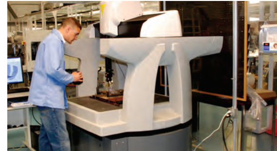
A measuring machine is adjacent to its medical molding cell to minimize the time required for first article inspections on new medical molding programs.
