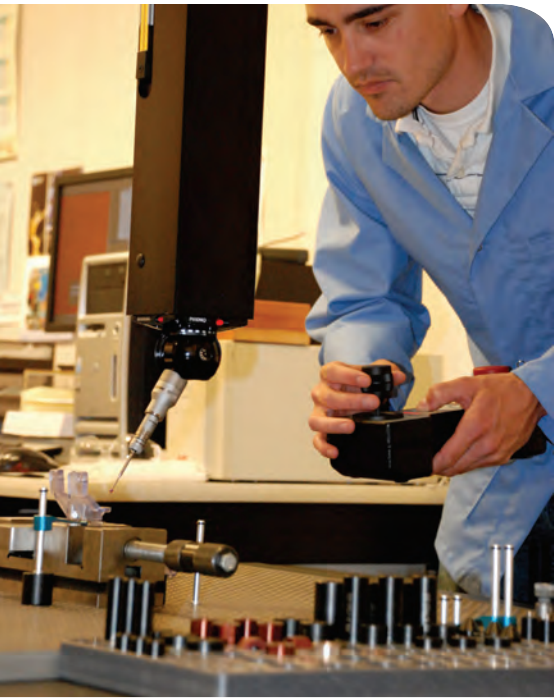
A metrologist conducts first article inspections, which consist of the measurement of all dimensional callouts on the molded product part print.
