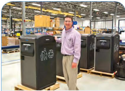
Arlington plant manager Bryan Campbell shows off one of Mack's contract manufacturing products—the Big Belly trash compactor, which includes 35 metal parts and a clear polycarbonate top.
