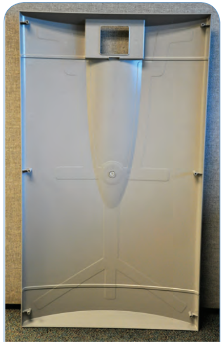
Mack favors external gas assist for its ability to save customers money by allowing use of smaller presses and simpler tooling to produce large-area parts with cosmetic surfaces—like this equipment cover measuring 46 x 26 in.
