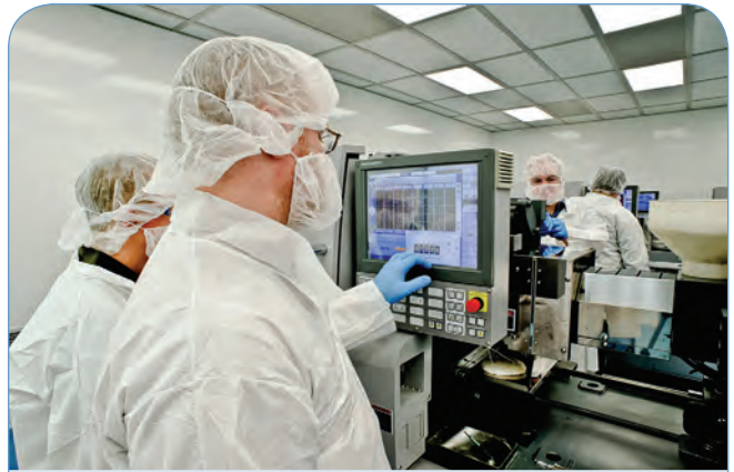
Supporting the growth of medical products as Mack’s top market segment, the firm installed its first permanent clean room this year. It houses six 110-ton, all-electric machines.
