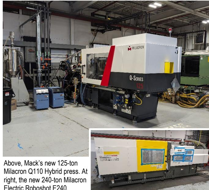
Above, Mack's new 125-ton Milacron Q110 Hybrid press. At right, the new 240-ton Milacron Electric Roboshot E240.
